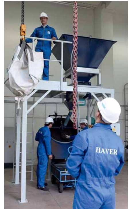
Pelletizing trials with concentrated iron ore on HAYER® Scarabaeus 1000-Pelletizing plate
