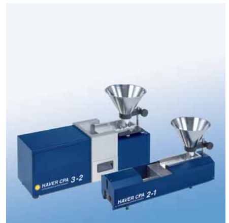
HAYER® CPA, photo-optic particle size and shape analysis
