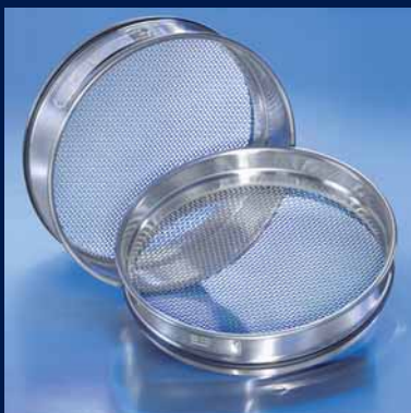
HAYER® analysis sieves for reproducible sieve analyses
