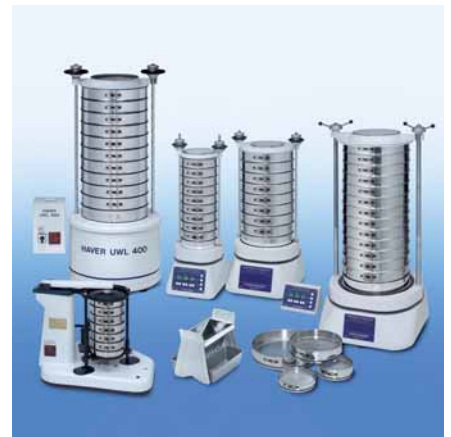
HAYER® sieve analysis machines with 3-dimensional screening movement and automatic amplitude control
