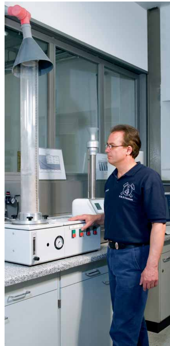
HAYER® DEAERATION TESTER with an exhaust hood with suction line
