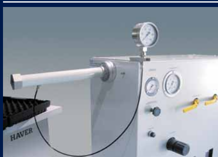
The HAVER® calibration unit allows annual testing of the HAVER® AIRFLOW TESTER's accuracy.
