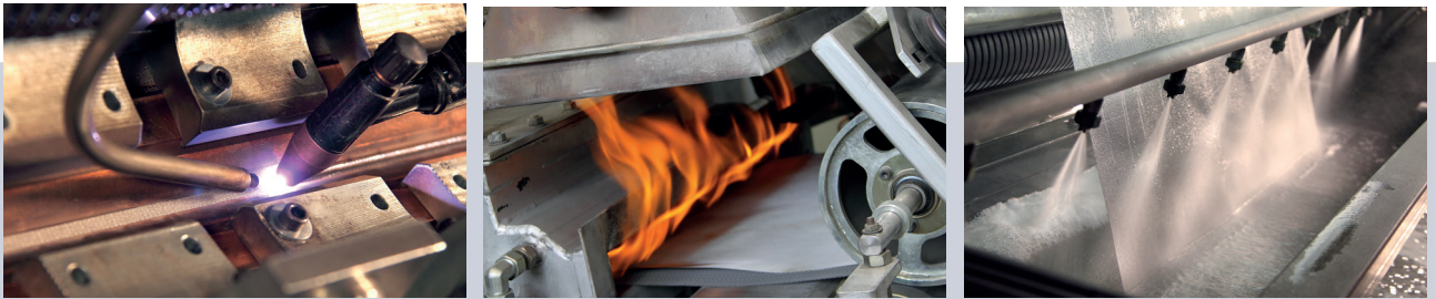
The production capabilities of Haver & Boecker include thermal treatment as well as welding and cleaning of complex filter elements.
